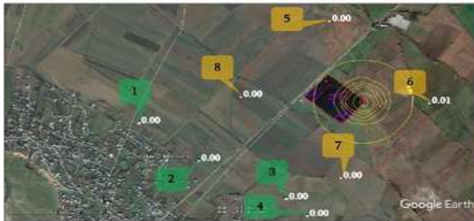
Maximum concentration of heavy fractions of saturated hydrocarbon (code 2754) at control points (nos. 1-4), at the nearest settlements and at the border of 500-m rated zone (nos. 5-8)
